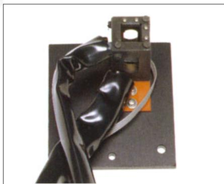
Keeps the sample at the desired constant temperature during measurement by circulating temperature-controlled water (5~70°C) around the sample cell. The stirring option has variable speed control and the minimum sample volume is 2mL. Effective for fluorometry of suspended cell samples.
