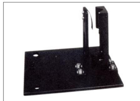
Holds a test tube, 12mm outer diameter and 60mm~100mm long.
