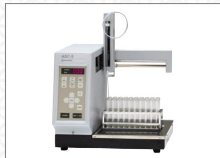
Builds an automatic multi sample spectrophotometry system in combination with a sipper unit. Up to 100 test tubes are set together on the rack. The aspirating nozzle is programmable to move X, Y and Z (vertical) direction.
