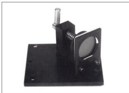
Provides a means to examine the fluorescence of a solid sample. The angle of the holder is designed to limit the reflected excitation beam from the emission monochromator. Standard accessories include a sample holder, quartz plate, powder sample plate, spacers and a sample fixing bar. Cutoff filters are included to reduce scattering further (UV-31, UV-35, UV-39, UV-Y43, UV-Y45, UV-Y47).
