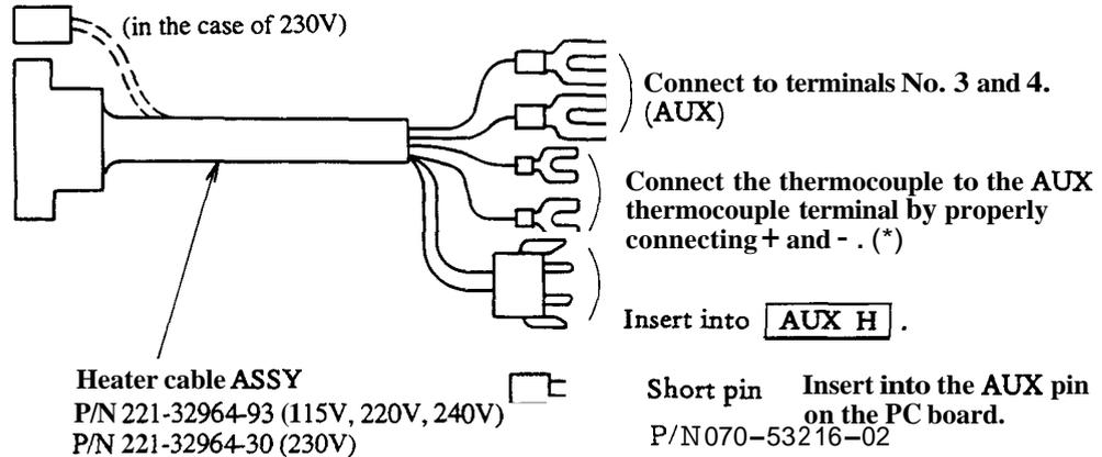
The most important thing for this operation is to correctly connect heater, heat sensor, and thermocouple to the PC board in accordance with the way shown. If they are not properly connected, temperature control does not function correctly causing excessive increase or decrease of temperature.
