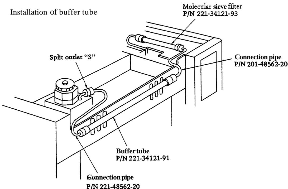
For installation of the buffer tube and the filter, use aluminium gaskets for column included in the standard accessory pack of Chromatograph main body. **This** filter is for protection of solenoid valve to control split ratio and needle valve. Remove the filter after injections of 50 to 100 times to check its contamination. To refresh the filter, put it in the column oven
