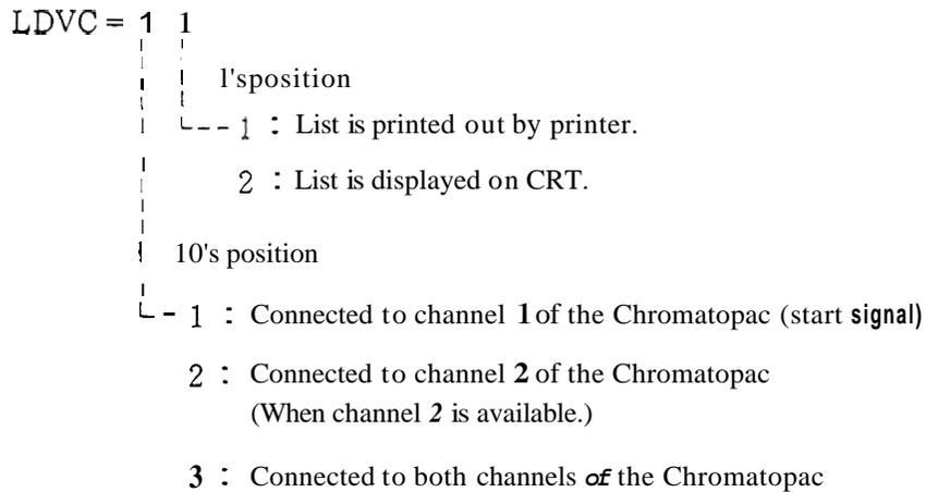
For instance, LDVC = 11 means that the list is output by the printer and the channel 1 of the Chromatopac is started up by pressing the **START** key of the **GC-14B**.
