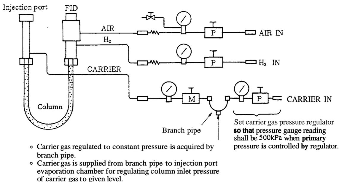
**Fig. 85 Application example for a packed column**
