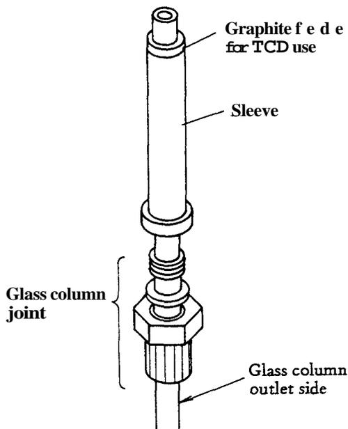
The TCD has no passage to purge the column outlet as in other detectors. With the FID, for instance, hydrogen gas enters at the column outlet to purge dead space.
