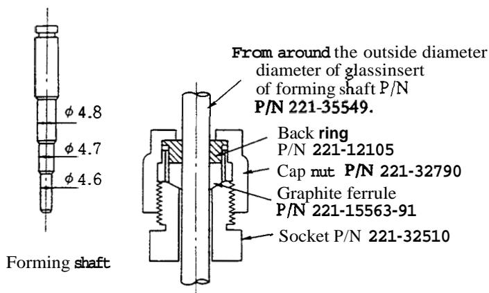
As shown in the above figure, put the graphite ferrule in the forming shaft and fasten its hexagonal nut with a spanner. Then, take out the graphite ferrule only and fix it in the glass insert.
