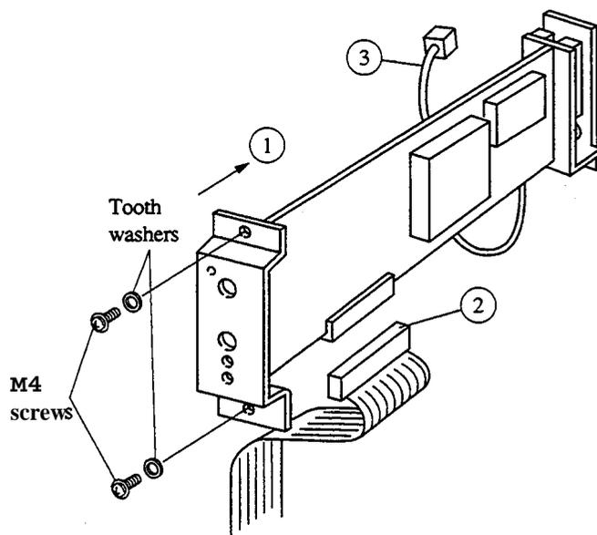
The TCD control unit is contained in the control unit casing at the right of the oven. Normally it is mounted in the 1st position.
