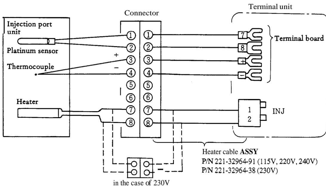
When installing or removing injection port units be certain the power switch is OFF before plugging/unplugging connectors. If done with the power switch ON, the CPU sees a disconnection of the circuit, thus actuating the protective circuit and automatically turning **all** heaters **OFF** at that point.
