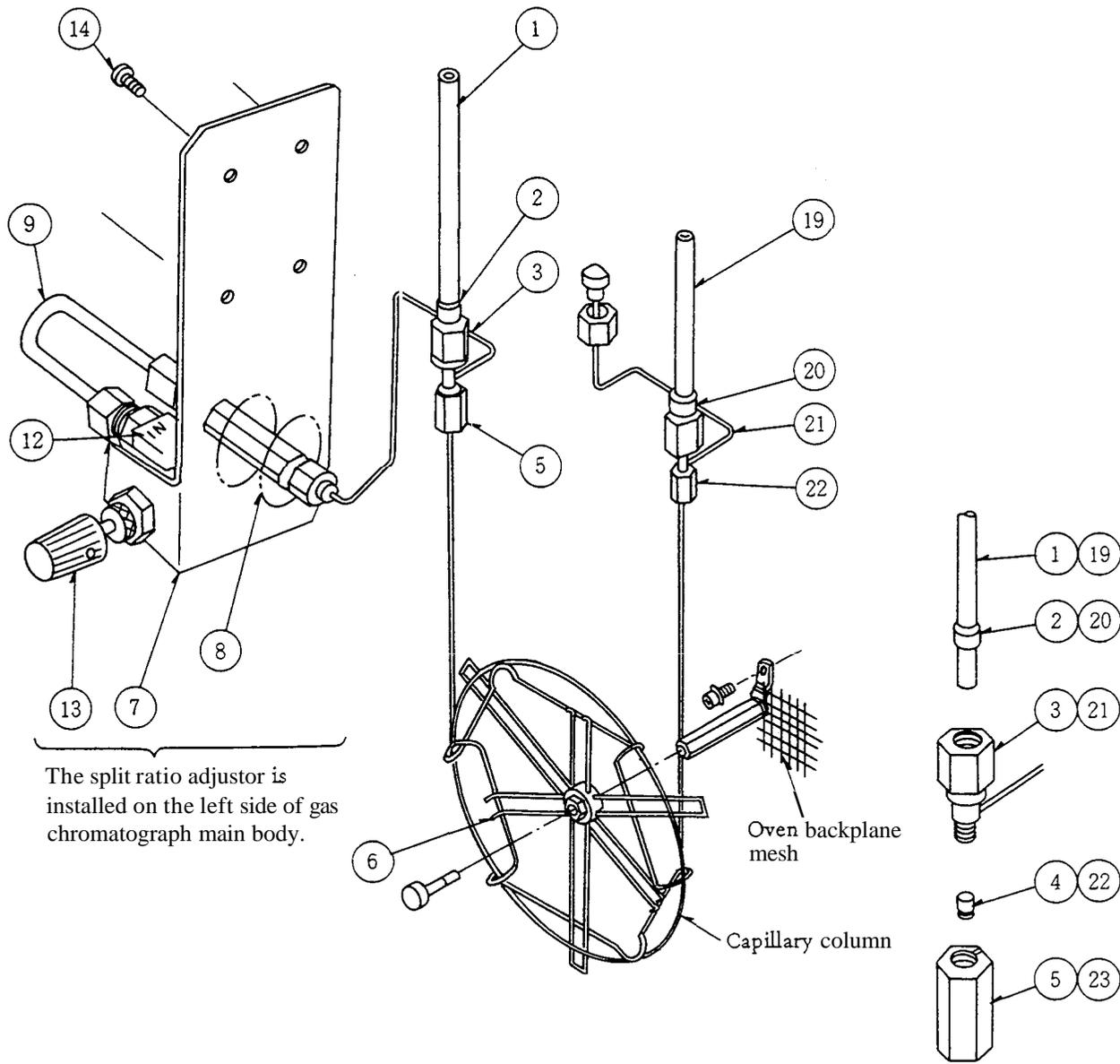
**Fig. 1 Construction of CLH-14 (No. 1)**
