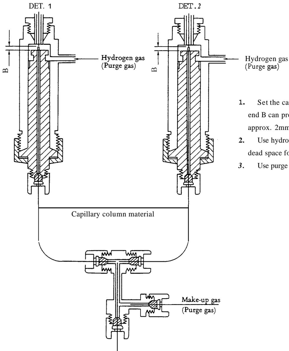
1. Set the capillary column so that its end B can project from the adaptor by approx. 2mm.
