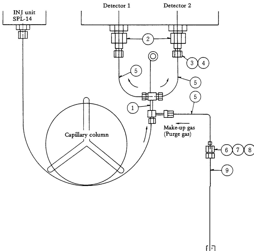
Detector-side branch parts set P/N 221-33495-91
