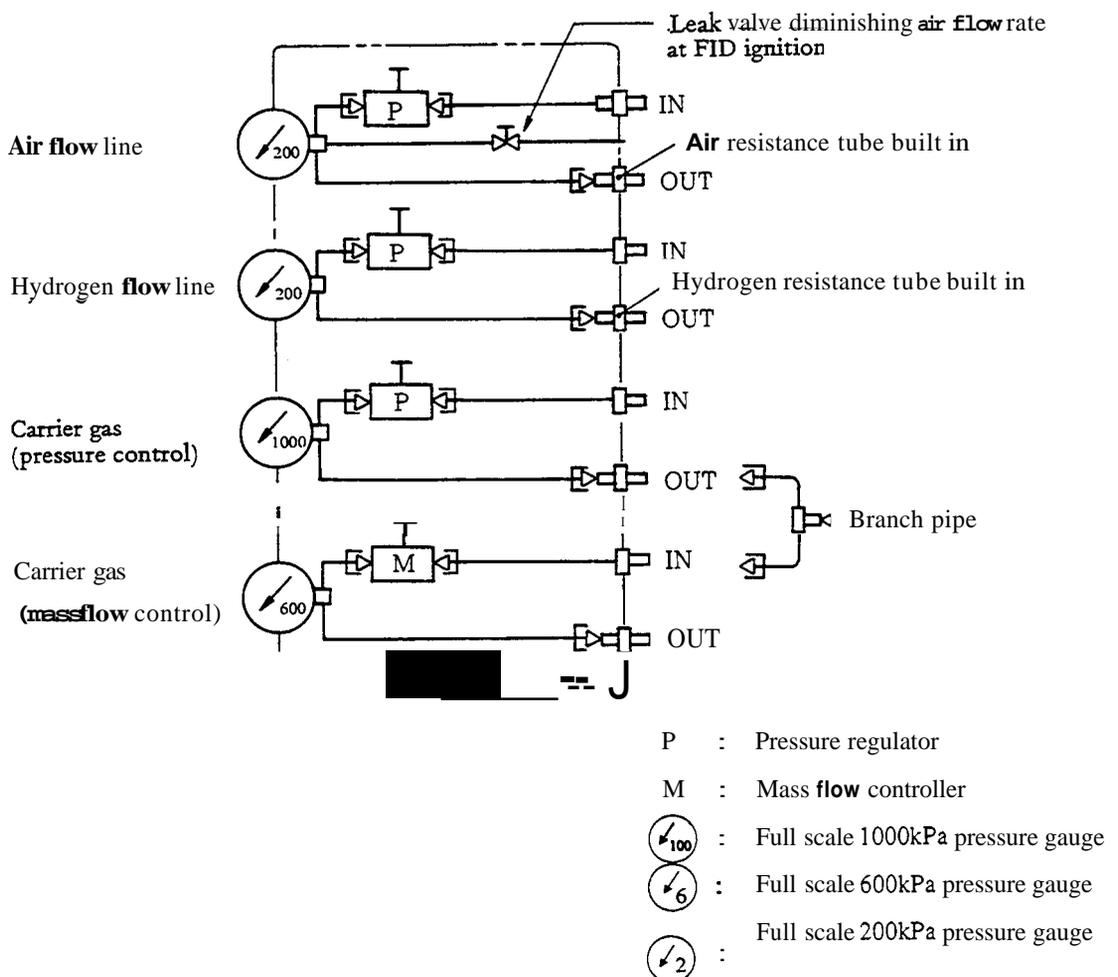
Fig. 84B Flow line diagram
