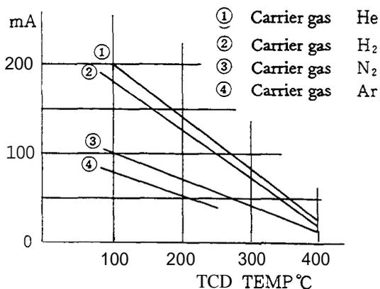
Current can be set from 0mA to 100mA in steps of 1mA. The upper limit of current supplied to the TCD filament differs, as shown in the figure at left, depending on the carrier gas type and TCD thermostatic oven temperature setting.
