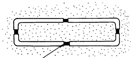
Cut the plastic joints to open the feed through when necessary.
