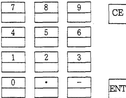
The range of figures that can be entered for display is up to **4** digits to the left of the decimal point and up to two digits to the right of the decimal point. If the integer portion of a figure entered exceeds four digits, the excess integer(s) becomes invalid. In the same way, if the decimal portion of a figure entered should exceed two digits to the right of the decimal point, the excess digit(s) becomes invalid.
