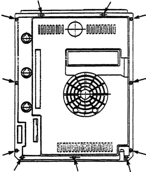
To detach the rear panel, first disconnect wiring for the detector control unit and for the optional boards.
