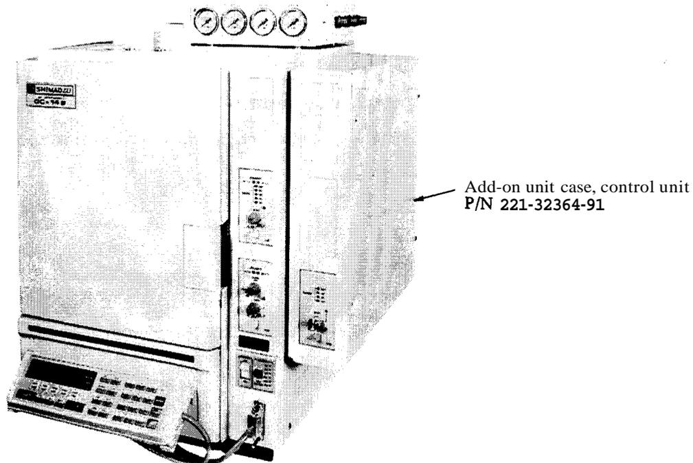
FIX the ground wire of add-on unit case to the rear panel of **GC-14B** as following figure.
