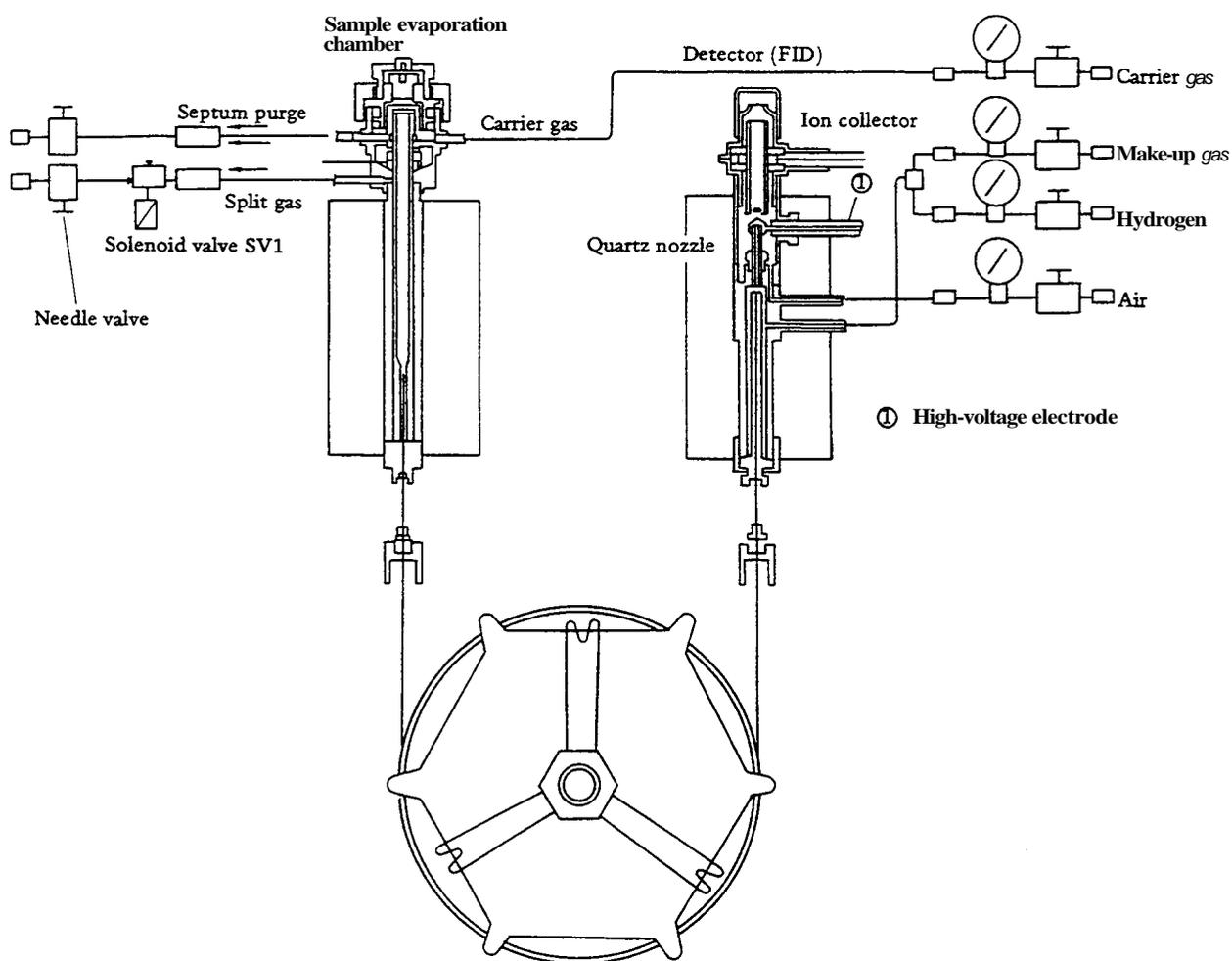
Fig. 7.1 Split/splitless sample injection method
