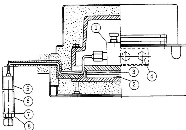
TCD cell ① is cased in the thermally controlled aluminium block. The inlet side of the TCD is connected from the lead pipe and column joint ⑤ to the column oven via the detector thermostatic oven.
