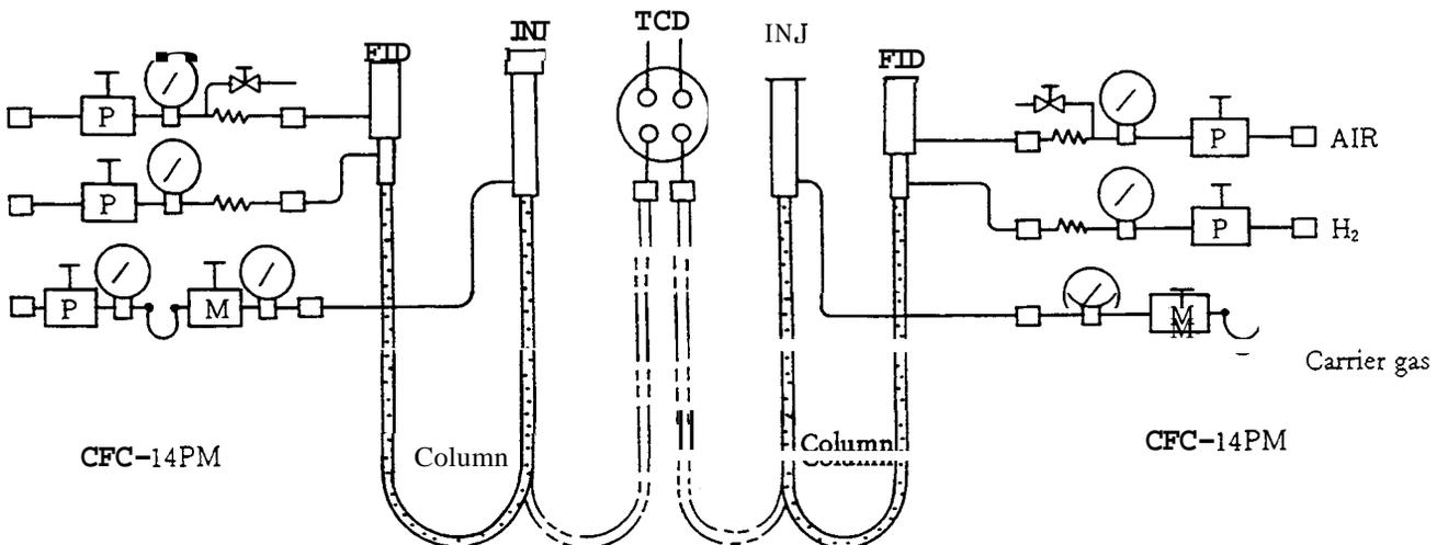
In dual flow line or dual column, two units of the flow controller CFC-14M are used to establish the complete dual flow line or dual column system.
