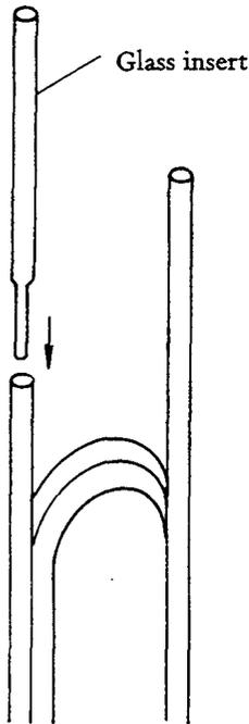
Inlet and outlet necks of the column are of different lengths. Insert the **glass** insert into the shorter neck, and set the assembly into the injection port.
