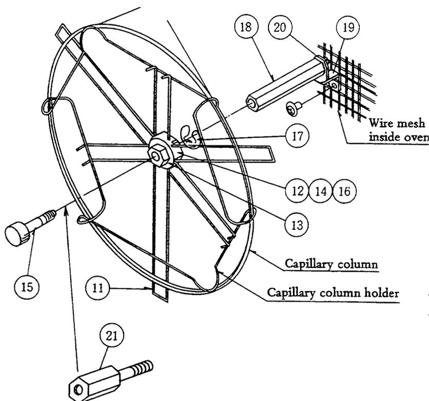
When two capillary holders are fixed, fix the first holder with this spacer and fix another holder to the threaded portion of the spacer.
