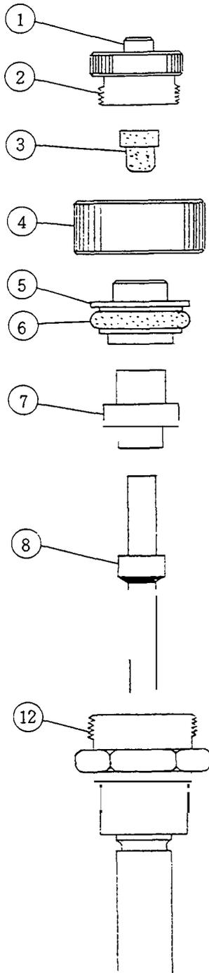
Remove nut (4) and pull seal ring (5) upward. Then, O-ring (6) is exposed. Replace the O-ring if it is worn.
