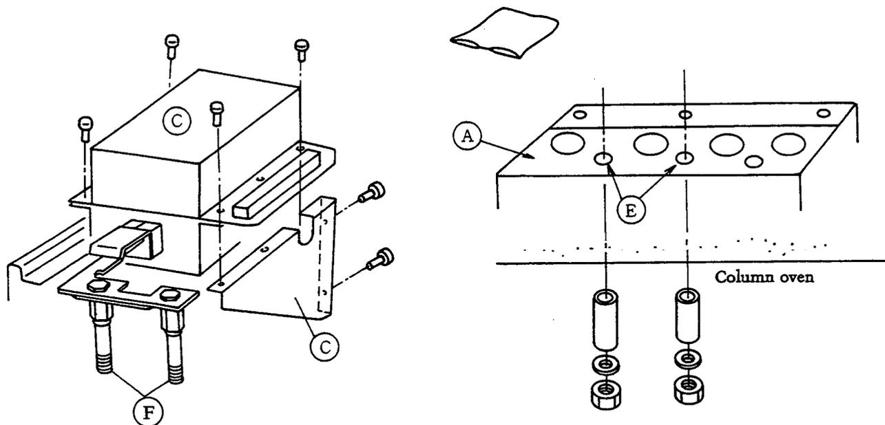
The TCD thermostatic oven is provided at the rear of the detector thermostatic oven at the upper part of the column oven.
