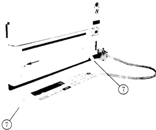
Insert the keyboard unit cable connector into the recess in the column oven as shown below. Observe the key on the connector. Tighten the two knurled screws firmly.
