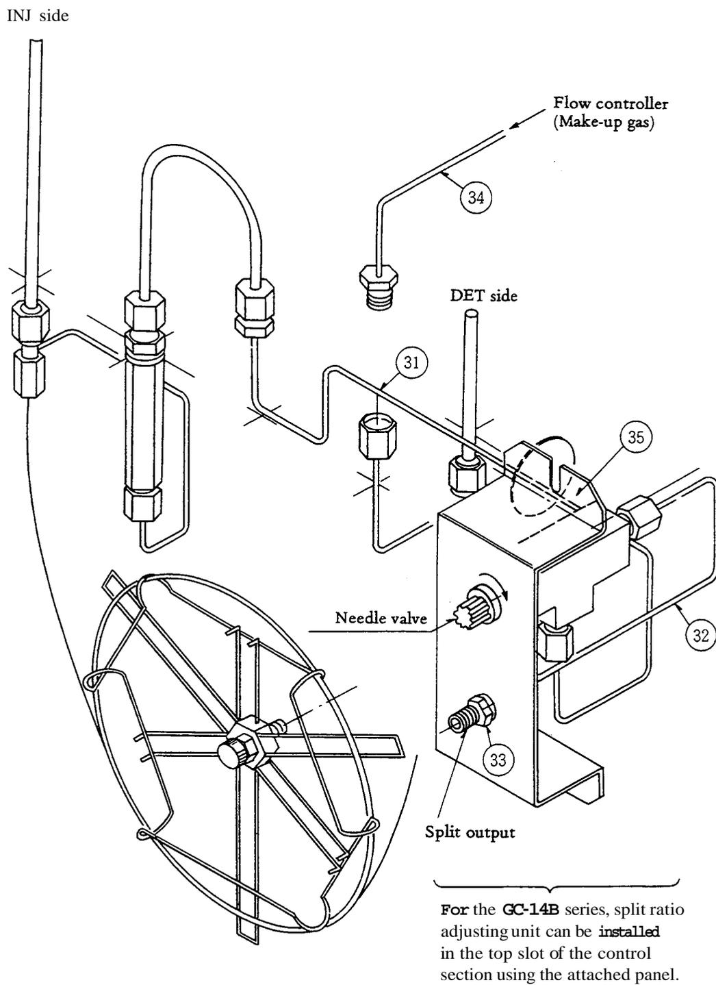
**Fig. 2 Construction of CLH-14 (No. 2)**
