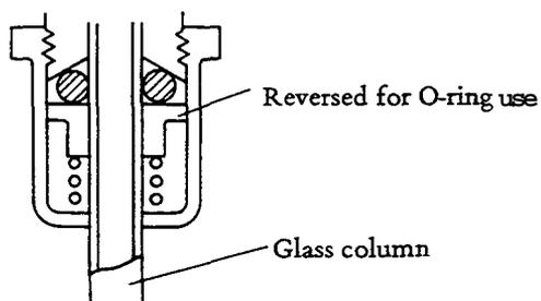
2. Although O-rings can be used easily, **all** O-rings have certain heat-resistance limits. Observe the limit for the **type** of O-ring used to prevent elution **of** compounds which **will** cause ghost peaks.
