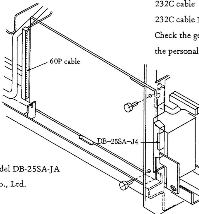
\*Connector Model DB-25SA-JA from Hirose Co., Ltd.
