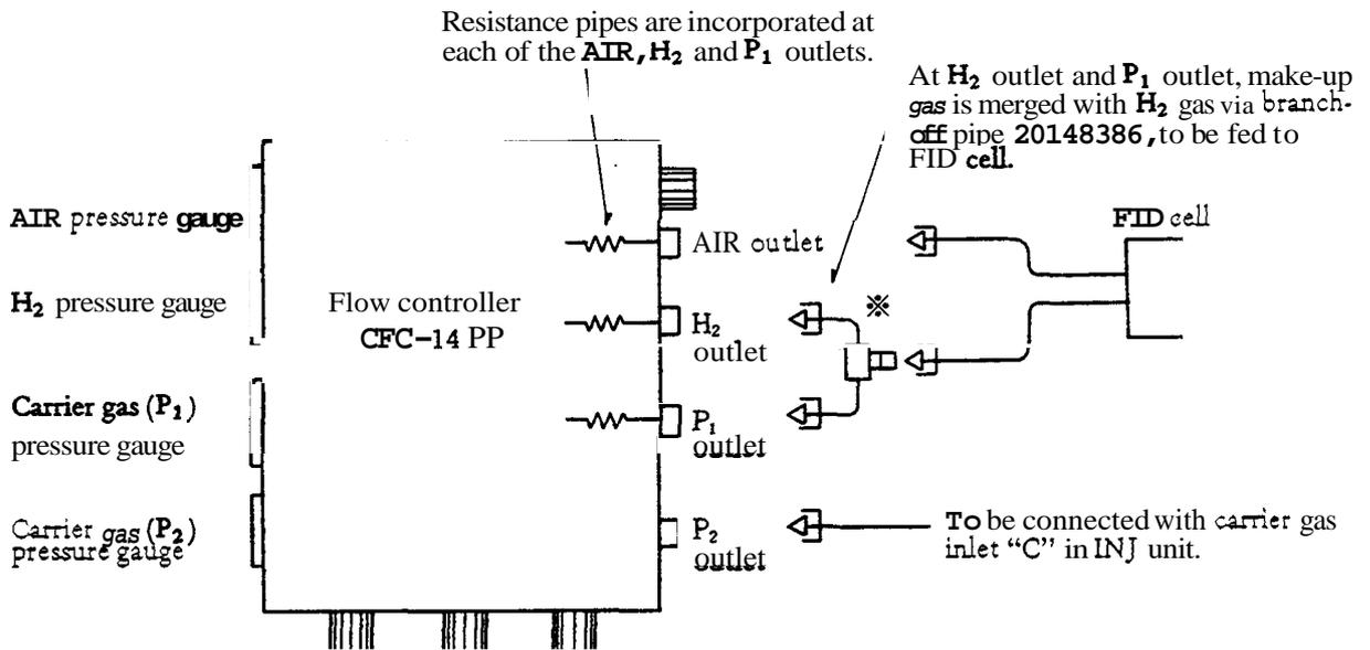
\* Before setting this make-up gas branch-off pipe, check reading on the P<sub>1</sub> pressure gauge and the quantity of make-up gas fed to the P<sub>1</sub> outlet. (Flow rate of about 40ml/min can be obtained with N<sub>2</sub> gas when the pressure gauge indicates 50kPa.)
