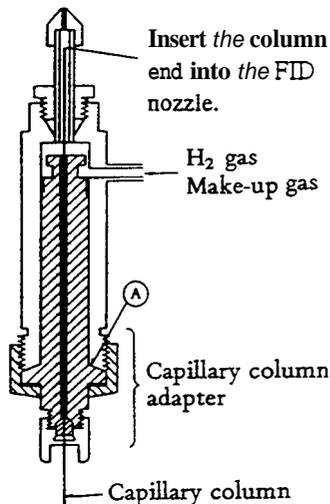
The capillary column is attached in metal-to-metal contact (without using any gasket).
