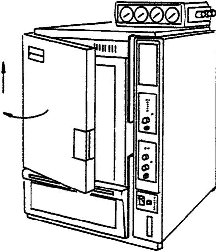
To dismantle the column oven door, open the door and raise the whole assembly to dismount the door.
