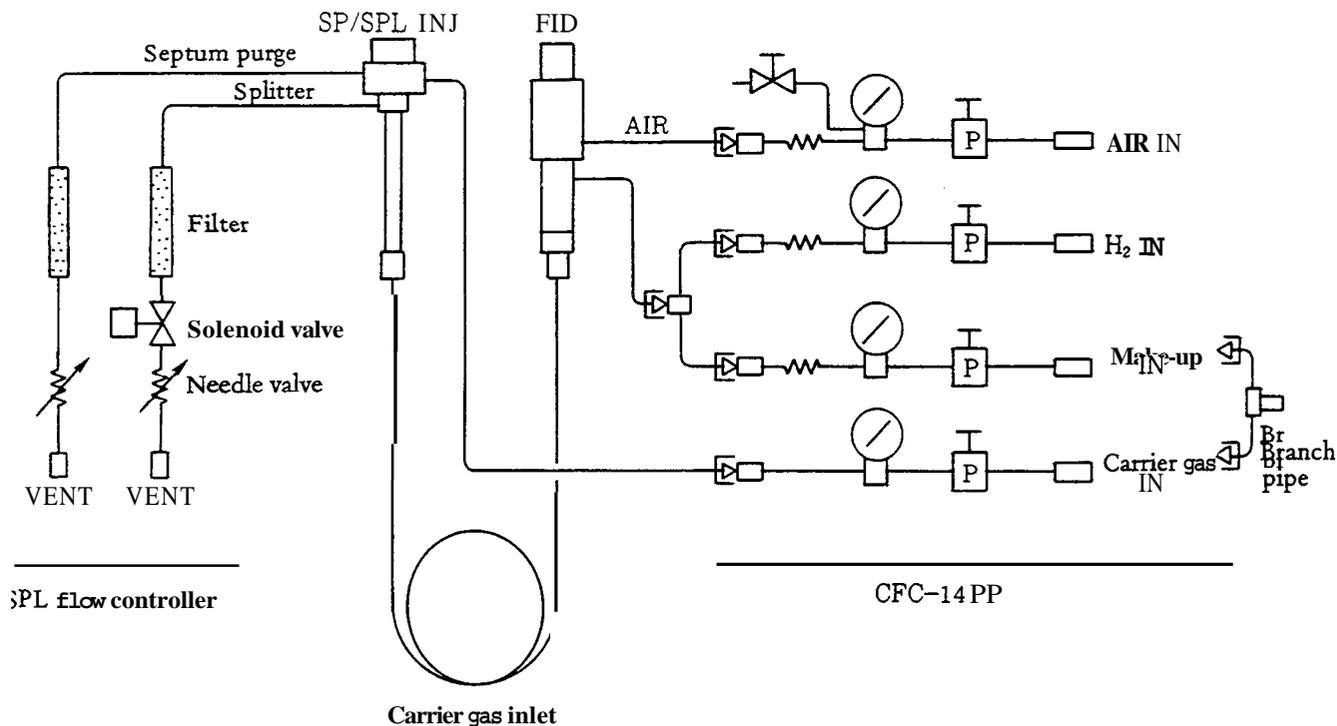
**Fig. 89 Application example for capillary column**
