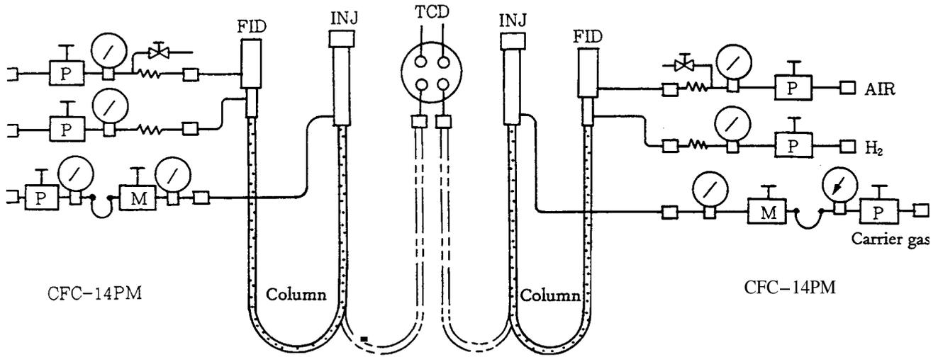
**Fig. 87 Application for dual columns**
