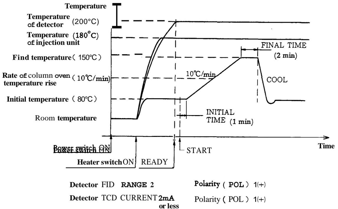
Fig. 32 Example of Condition Setting for Operation Check
