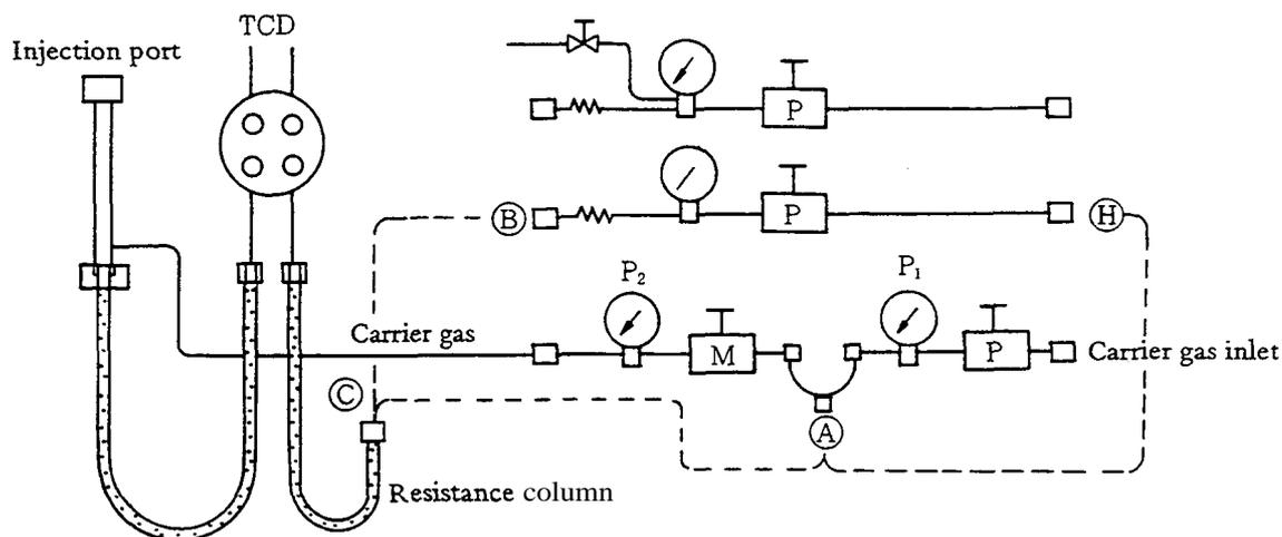
**Fig. 86 Application example to packed column and TCD**
