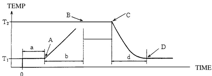
Parameters necessary to prepare the single-step heating program of the heating pattern shown above are as follows:
