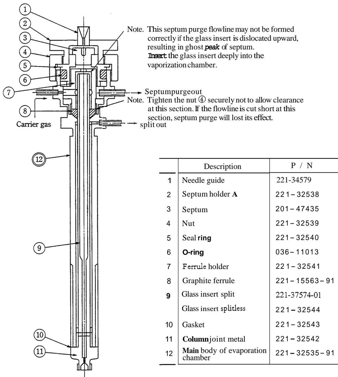
**Fig. 7.10 Injection port of SPL-14**
