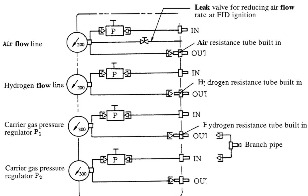
Fig. 88B Example of flow lines
