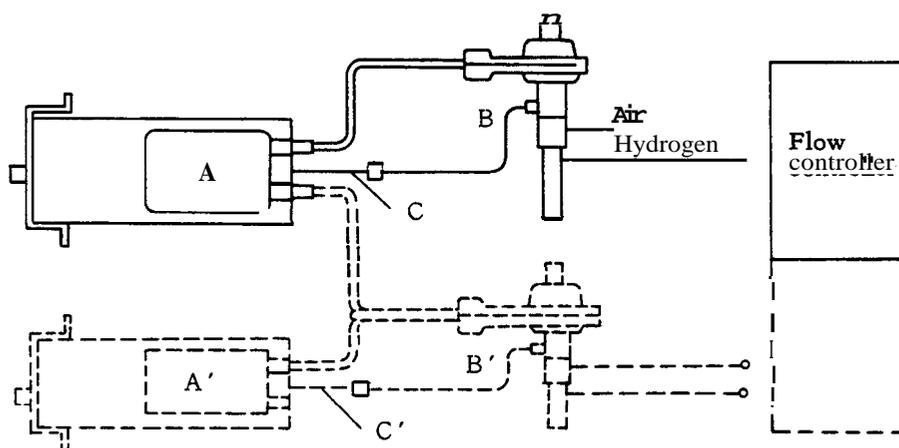
**A:** FID control unit (Electrometer) P/N 221-23820-96 (for 230V)
