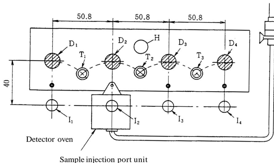
The diagram above is the top view of the detector section.
