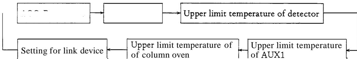
It should be noted, however, that the function for requesting listing of parameters to the Chromatopac and the function of self-diagnosis are not included in this circular list and cannot be selected no matter how many times the ENT key is pressed.
