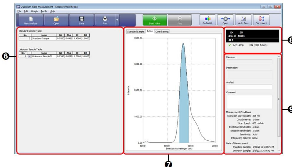
Window Layout of the Main Window (Measurement Mode)
