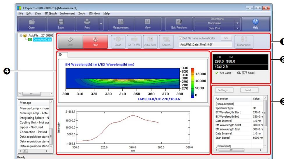
Window Layout of the 3D Spectrum Application (Measurement Mode)
