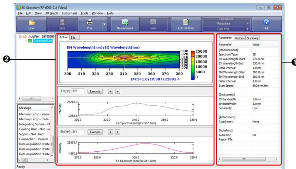
Window Layout of the 3D Spectrum Application (View Mode)
